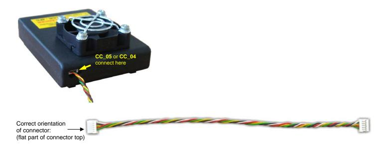
Connect the needed number of balancers (here three) through CM-3 module using CC\_05 cables. 2 or more cells (see instructions for use BLCR 4FC or BLCR 5FC) to each balancer. To connect the PC, connect CM-3 module to USBCOM+ using cable CC\_03.
