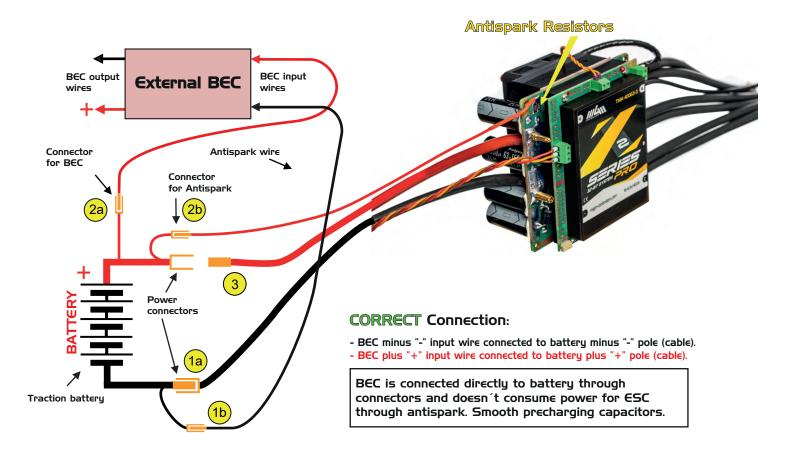
Correct procedure of connecting ESC and BEC with traction battery
