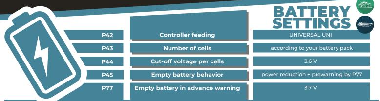
Recommended settings for LI-PO batteries (for cars and boats). You will prevent possible damage to your batteries by setting these parameters correctly.
