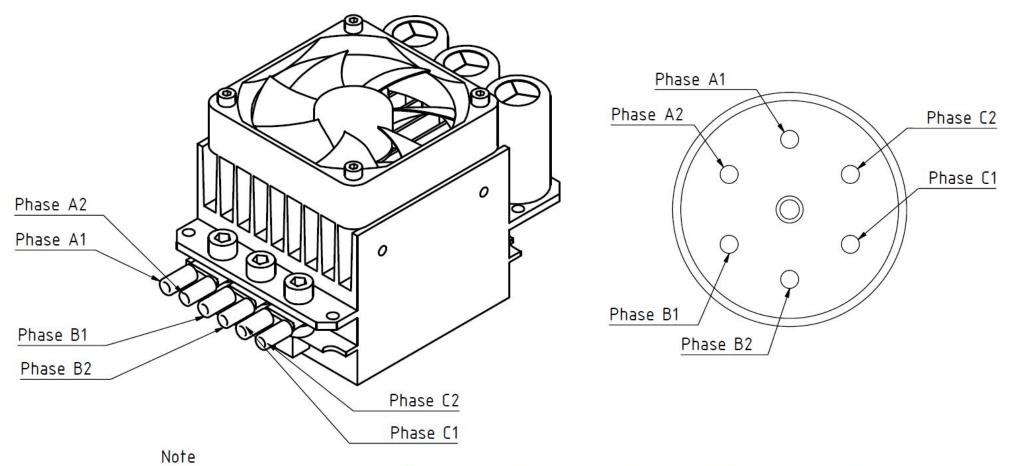
If motor rotates in reverse, please change the wires of Phase A with the wires of Phase B.
